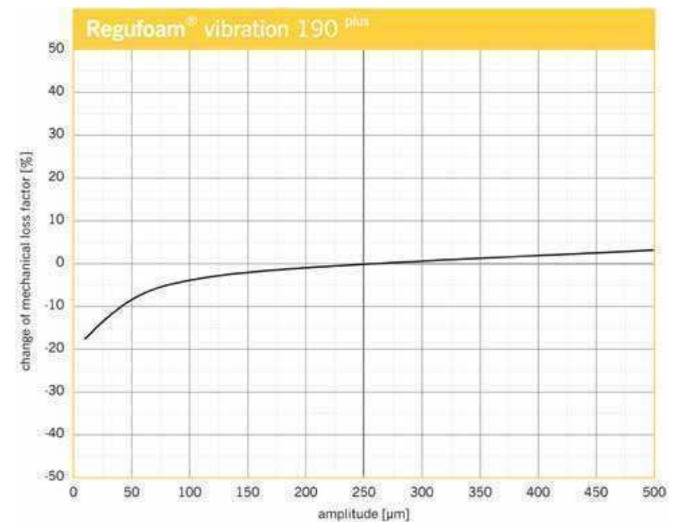
Change of the mechanical loss factor due to changes in amplitudes. Sinusoidal excitation at a constant mean load of 0.018 N/mm 2 , dimensions of the specimens 300 mm x 300 mm x 25 mm.
